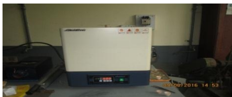
(A). Ashing samples in furnace
